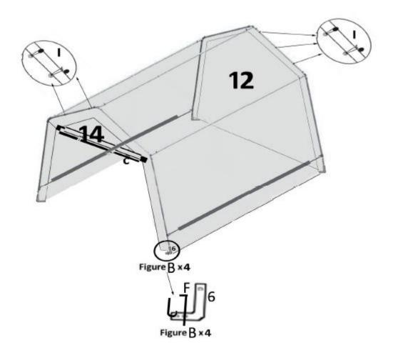
TOP TIP: Place the four bottom corners of the front and rear doors under the base tube to prevent it from moving:
