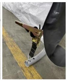
2. Before completely tightening, insert the hook in the hole at the end of the base tubes (6), and continue tightening the roof fastener until you have the desired tension on the roof.
