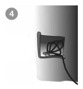
Place the pump and excess wires into the access cavity, ensuring that the long pump and LED wires extend out through the opening
