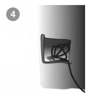
Place the pump and excess wires into the access cavity, ensuring that the long pump and LED wires extend out through the opening
