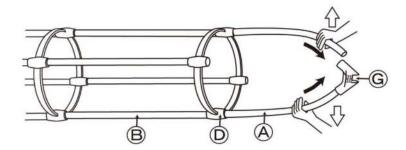
4. Continue connecting the 2 bends (A) with the whole structure, secured by connector 1 (F) and the connector 2 (G), push them together.
