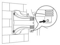
(5) Optional- The hose reel can be securely locked to the bracket by placing a padlock (not included) through the hole of the pin under the bracket.
