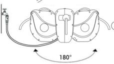
Attach the tap to reel connector to your tap using the universal tap adaptor. Test to ensure the reel rotates freely through 180°
