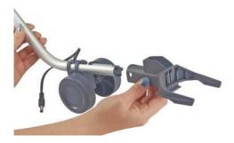
3. Attach the trimming shears to the mount, then connect the cable.
